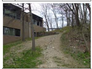
Photo Recommend installing concrete steps at #160: rear leading to front main entrance (southeast corner of building)
