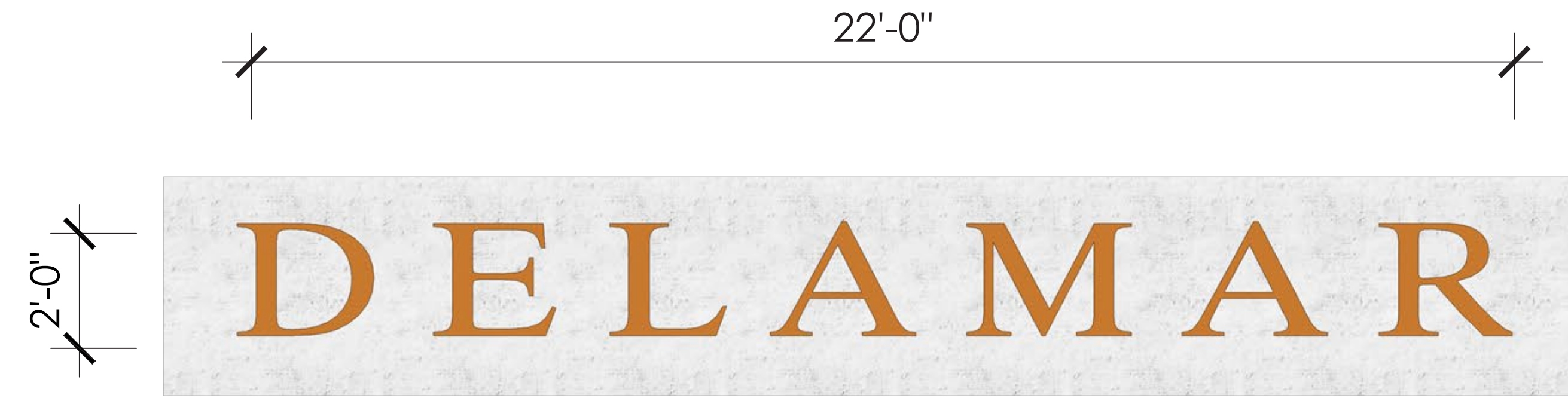
01 - BUILDING & RESIDENCE SIGN - HALO LIT METAL LETTERING IN GOLD FINISH 2'-0" X 22'-0" = 44 sqft SCALE: 1/2" = 1'-0"
