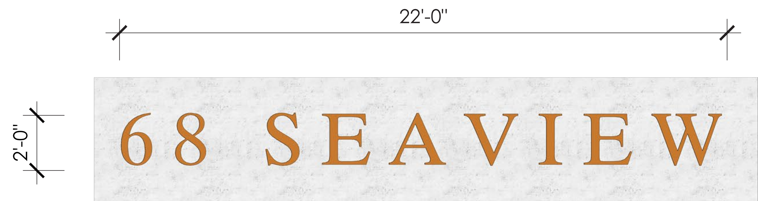
03 - MARINA ADDRESS SIGN - HALO LIT METAL LETTERING IN GOLD FINISH 2'-0" X 22'-0" = 44 sqft SCALE: 1/2" = 1'-0"
