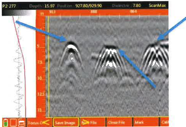
GPR data screenshot of more PT cables found in the rec room. All arrows point to PT cables
