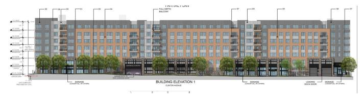
**View of Block B along Clinton Avenue** - The proposed buildings have brown brick masonry along the base of the building. This feature distinguishes it from the downtown office buildings which use mainly glass and steel materials. The mid-section of the building uses earth-toned hardisiding. The top will use gray colored hardie-panels.
