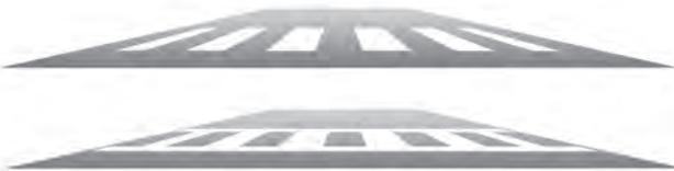
Standard crosswalk markings are composed of two parallel lines, which are virtually invisible from a distance compared to high visibility crosswalk markings. Thick striping perpendicular to the direction of the crossing allows drivers to more clearly see the crosswalk. This is because the perceived thickness of the long, perpendicular line is greater than that of the parallel line.
