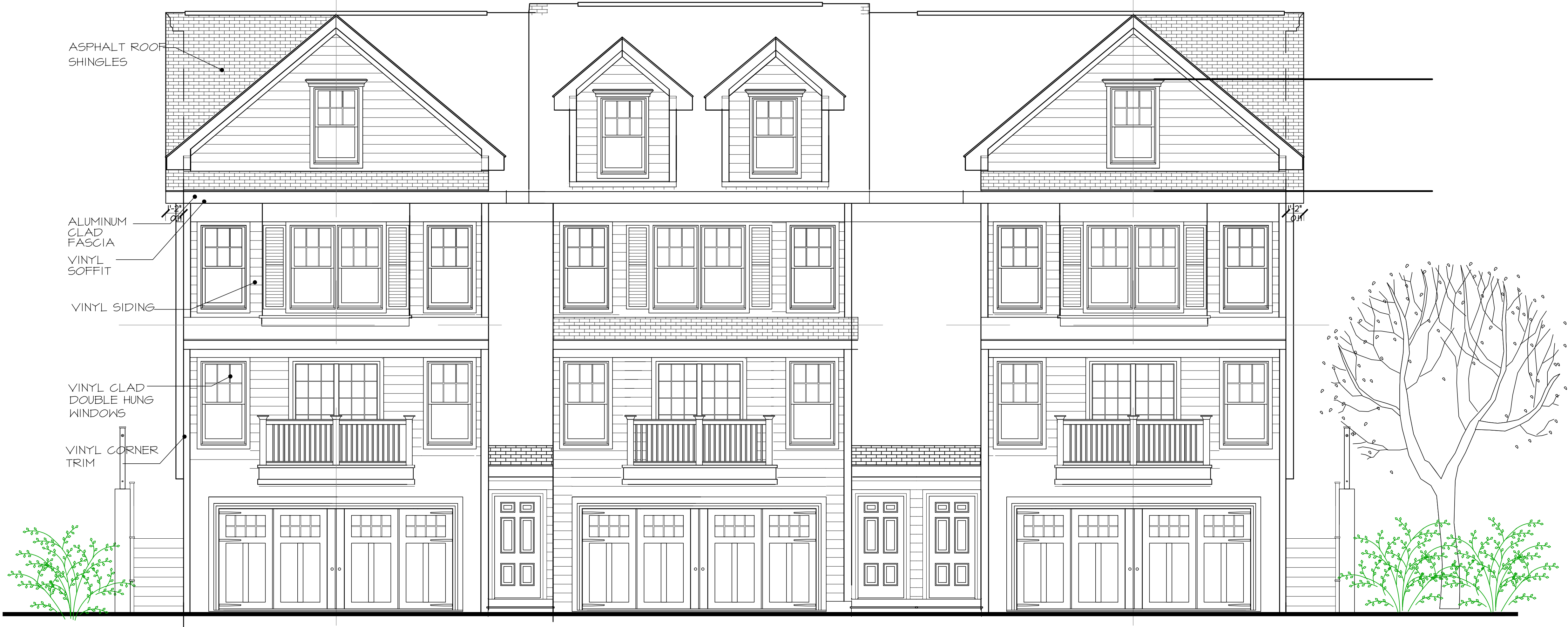
FRONT ELEVATION SCALE: 1/4"=1'-0"
