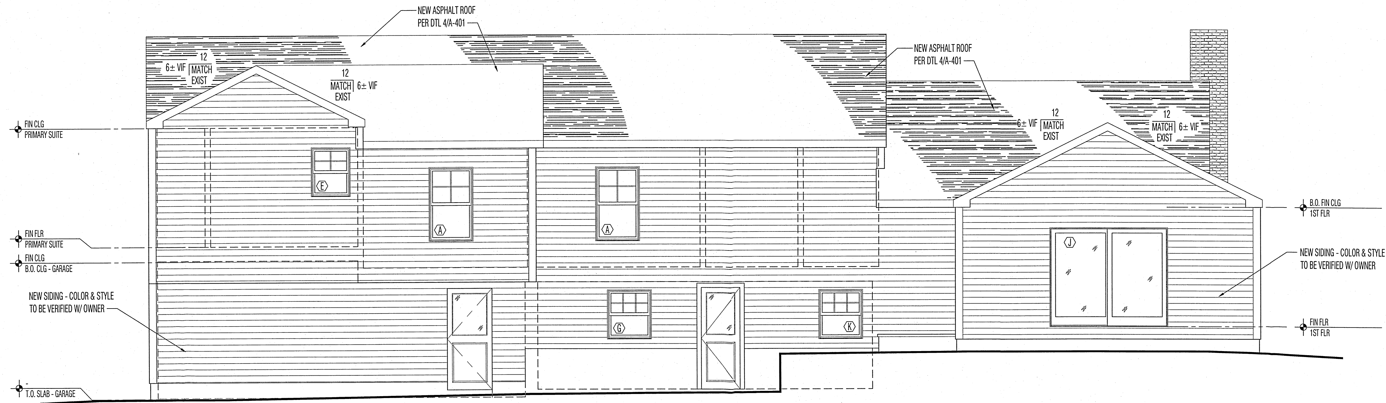
1 EXTERIOR ELEVATION - WEST FACING A-301 SCALE: 1/4" = 1'-0"
