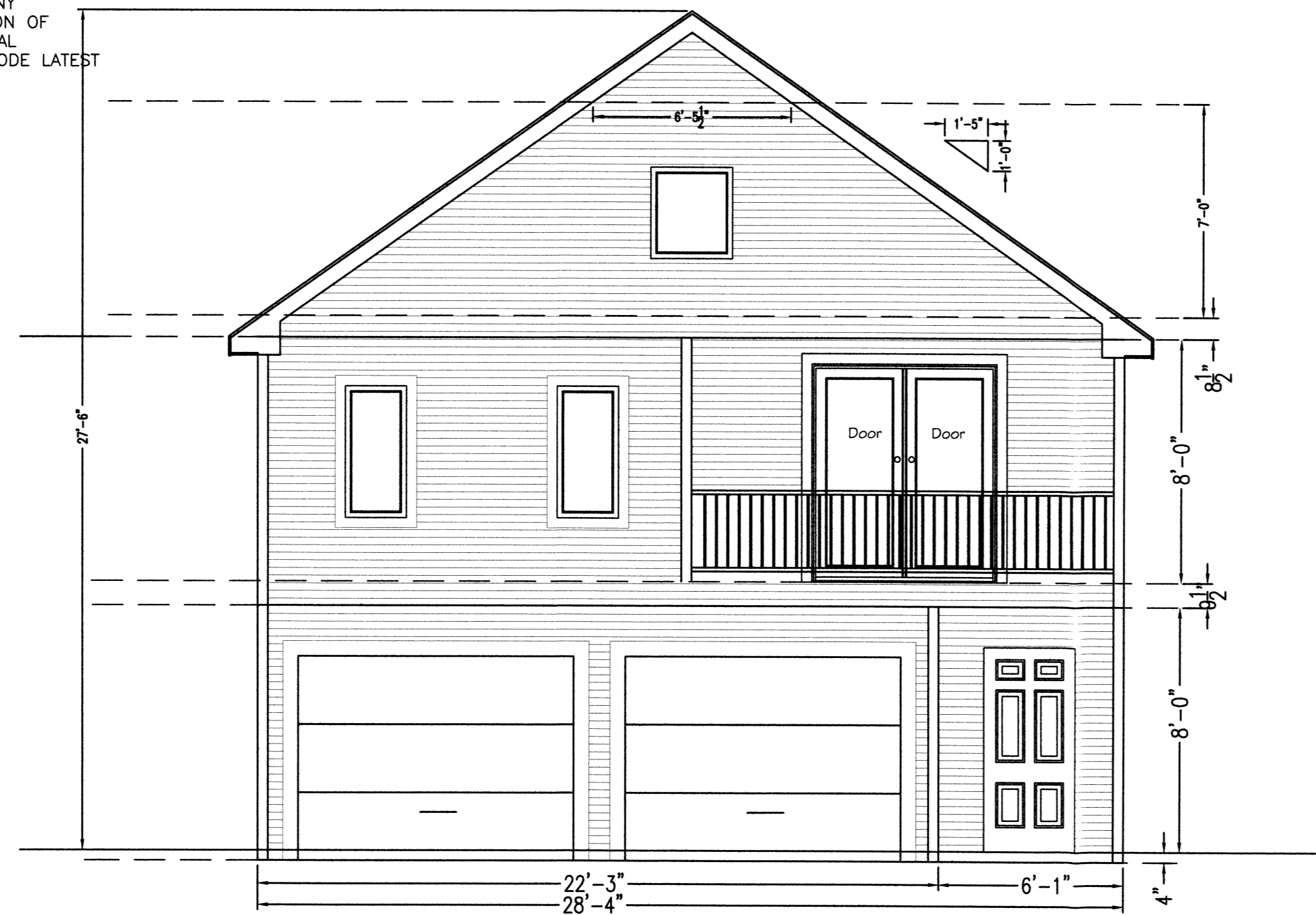
1 Proposed Front Elevation SCALE: 1/4" = 1'-0"
