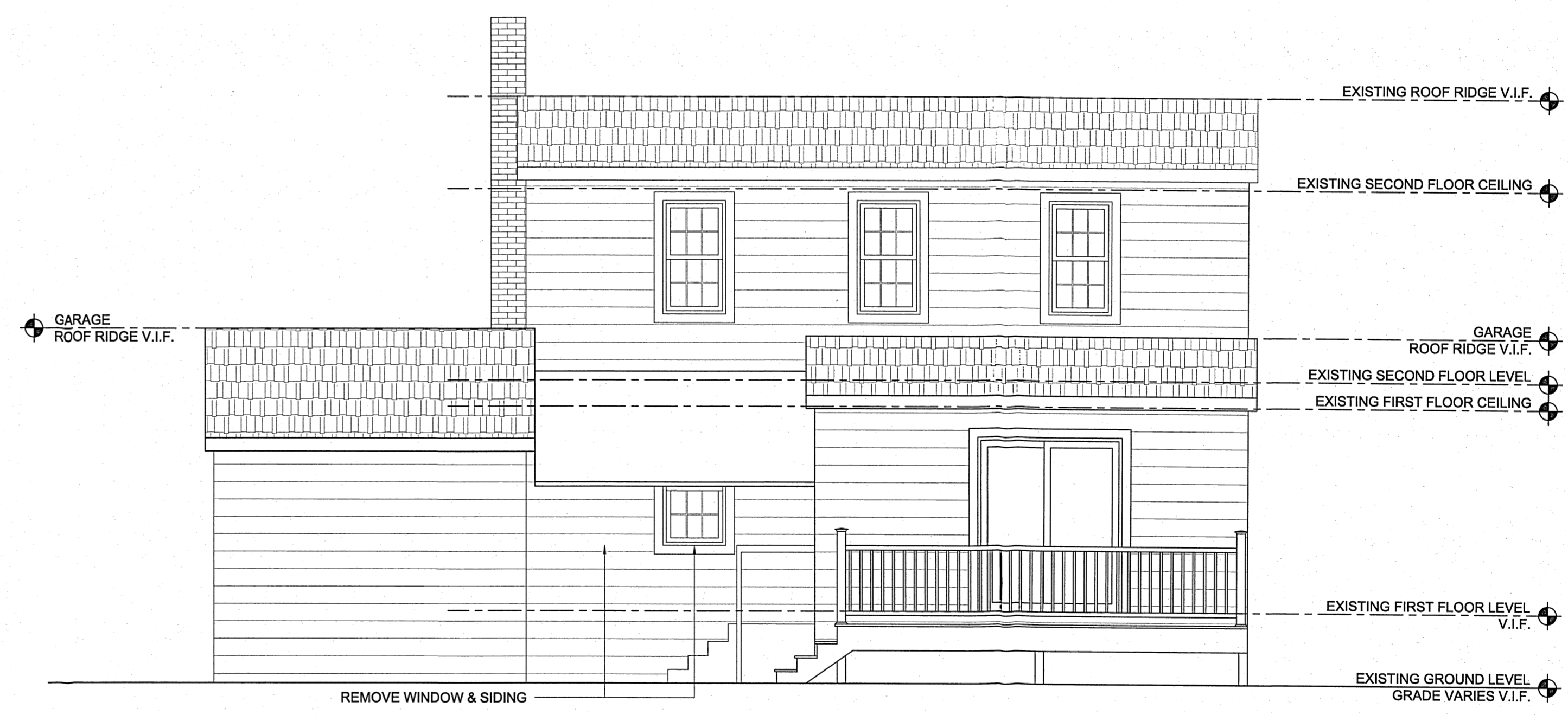
2 EXISTING / DEMOLITION WEST EXTERIOR ELEVATION SCALE: 1/4" = 1'-0"
