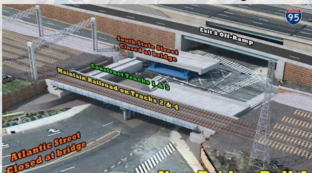
The bridge decks for the south side of the bridge are rolled into place right from the job site.
