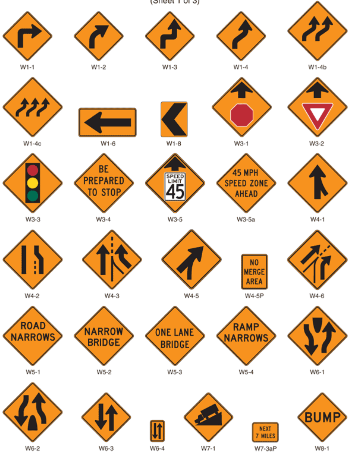
Figure 6F-4. Warning Signs and Plaques in Temporary Traffic Control Zones (Sheet 1 of 3)
